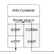
Figure 2: Example of a SOAP/HTTP-to-CORBA Router
