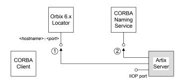
Figure 2: Artix Server Binding a Name to the Naming Service
