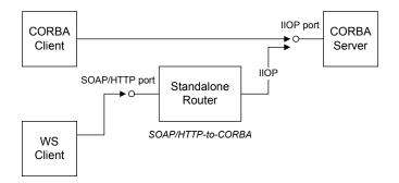
Figure 3: WS Client Accesses CORBA Server through Standalone Router
