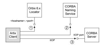
Figure 1: Artix Client Resolving a Name from the Naming Service
